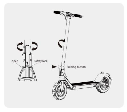
Step 2: Folding down the steering column, align the locking clasp with the side of the locking hook, then lock the steering column with the locking hook.
