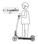
4. To slow down or stop the scooter, release trigger and hold the brake lever.
