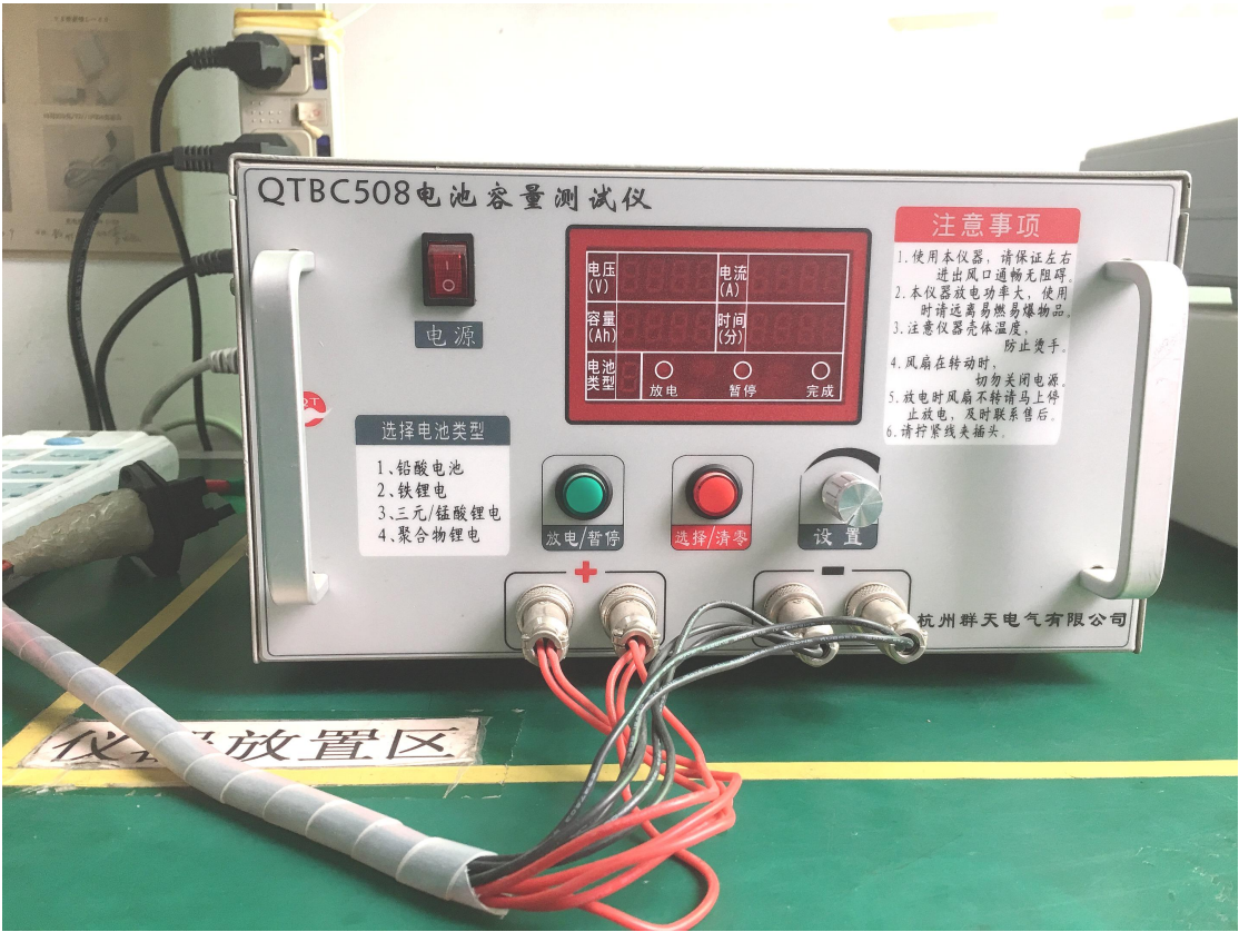
Battery capacity test
