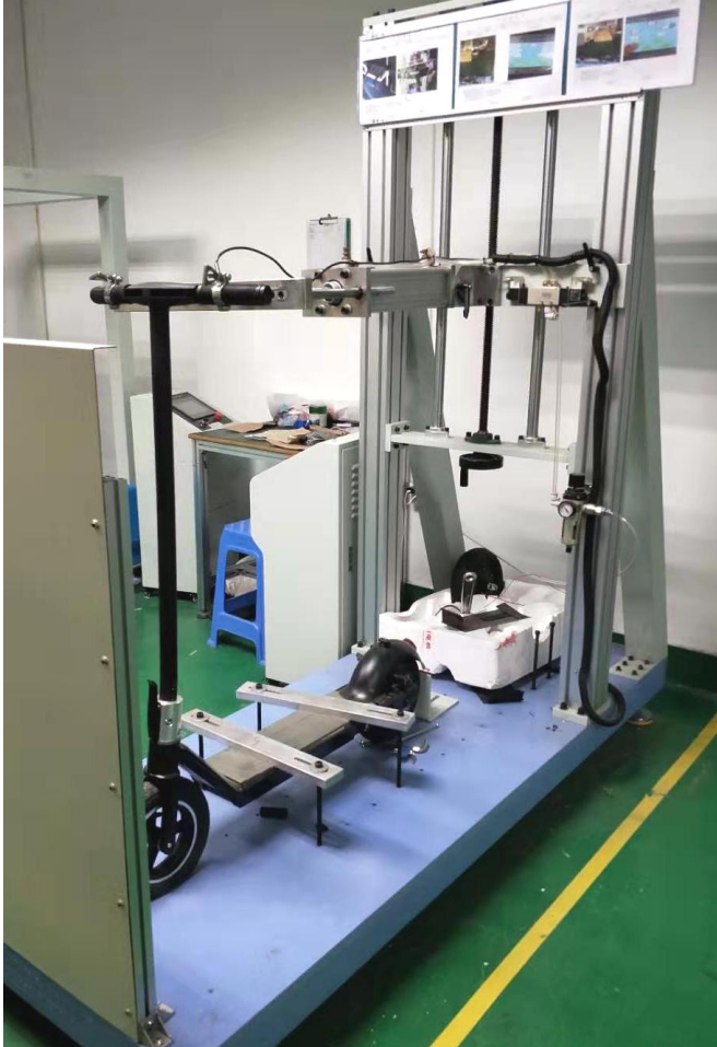
Strength test of the steering column
